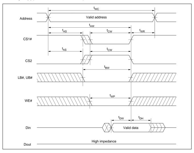
Write Cycle (2) (CS1#, CS2 Clock, OE# =  $V_{IH}$ )
